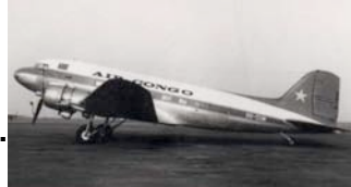
DC-3, Riveted Metal Structure, Retractable Gear
